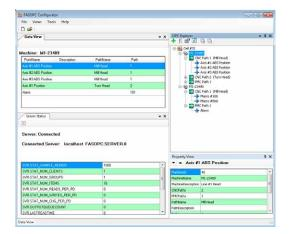
FASOPC supports most FOCAS enabled FANUC CNCs over Ethernet and HSSB.
